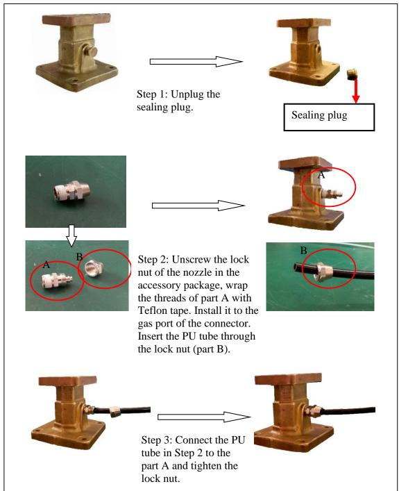
After connecting the tubing, make sure that the air path of the tubing between the dehydrator and the feeder system is unobstructed. Do not bend the tubing.
