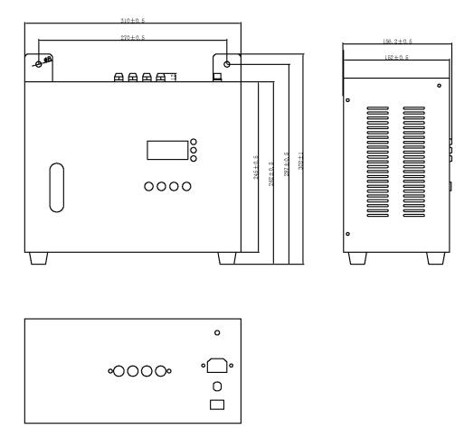
The dehydrator can be mounted on a wall using the supplied brackets. Following the hole location diagram shown in the figure.
