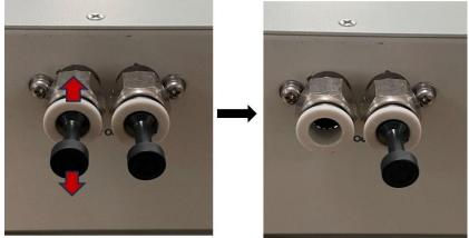
Switch on the power to activate the dehydrator and let it run for 3-5 minutes with nothing attached to the dry air outlet fitting. Check the airflow coming from the gas outlet using your finger. Disregard any alarms shown on the front panel.
